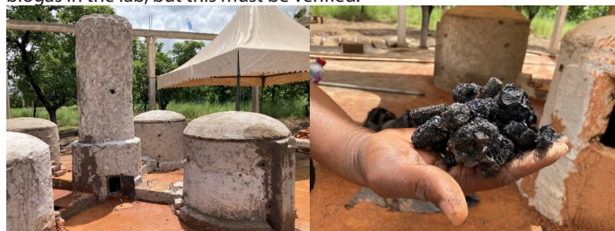
Figure 1 Newly constructed Brazilian kiln with four chambers and common chimney and resulting corn cob biochar in Loagri, Ghana
