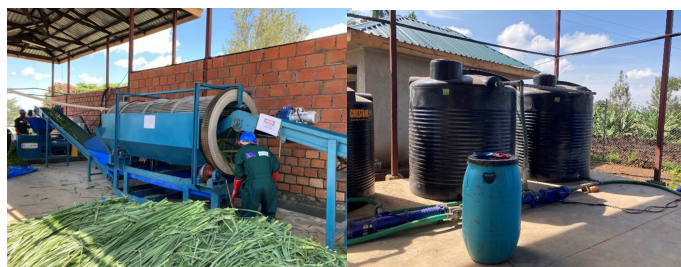
Figure 2 Protein refinery in Fort Portal, Uganda. Left washing of leaves, right tanks for protein coagulation and whey
